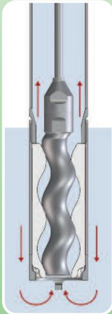
Removal principle of eccentric screw pump as an immersion pump
