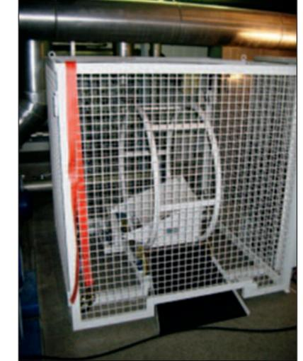
Fig. 5: Drum hoop mixer for homogenising the CO<sub>2</sub> extract
