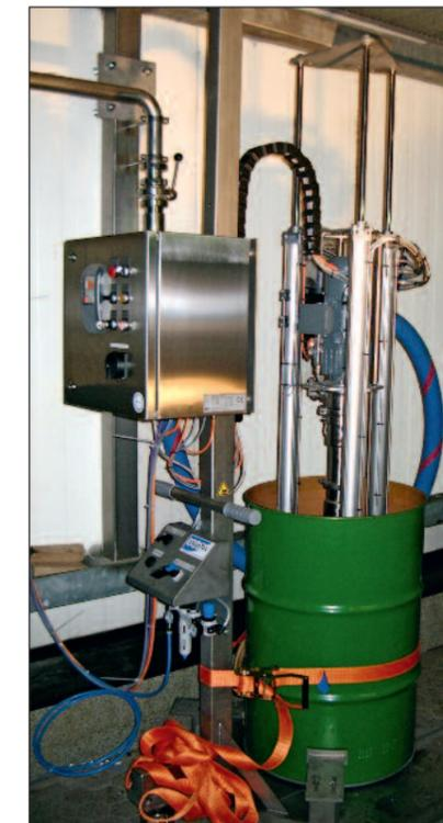
Fig. 1: The equipment comprises a frame with pneumatics, an eccentric screw pump with following plate and a parametrised frequency transformer with Profibus Module.
